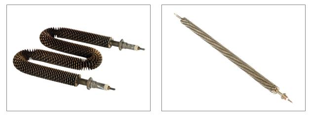
This type of heating element from Cato-Tech A/S is supplied as a component for duct heaters. Length can be changed according to the duct size and baffles; may be mounted to avoid duct vibrations.
